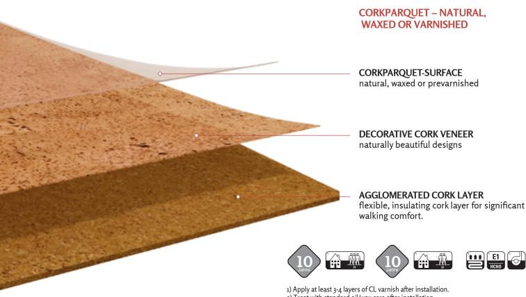
a) Apply at least 3-4 layers of CL varinsh after installation.
